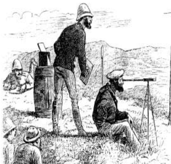
Beddoes' method, with sighting rods
